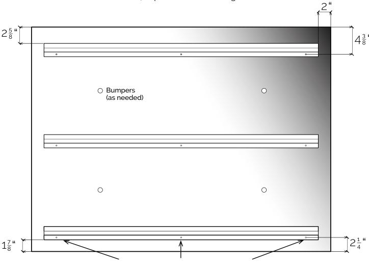
Installer to drill 3/16" holes in top and bottom wall brackets within 2" of end of bracket (max). Other drillings to align with studs whenever possible.
